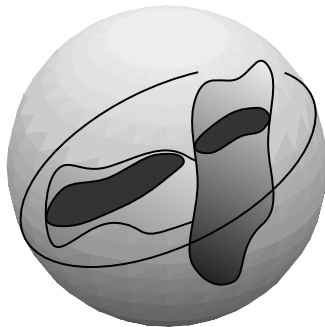
Fakir probe (classical motion invariant test lines)
